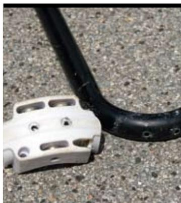
❶ Remove the old cleat by drilling through the blind rivets. If they start to spin, show them no mercy – use a screwdriver or awl to remove them.
