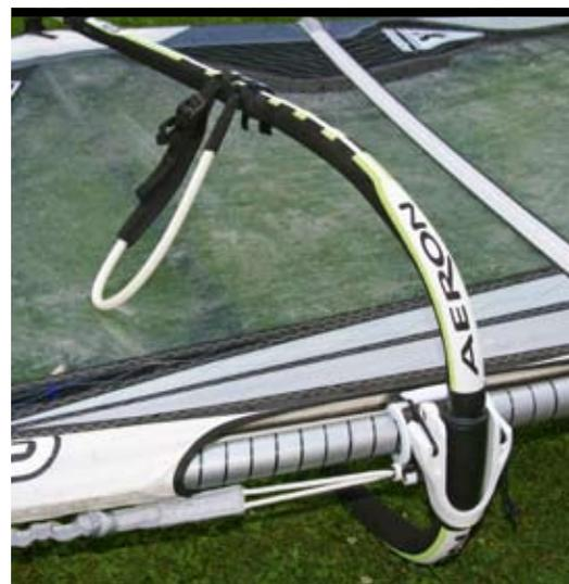
❶ If your boom has a clamp that closes under the mast, which makes it difficult to rig, just turn the boom around!
